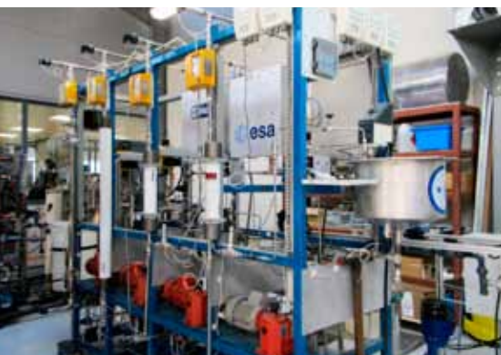
PROTOTYPE ESA – GREY WATER TREATMENT UNIT
