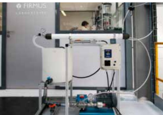
PILOTE FIRMUS NANOFILTRATION – OSMOSE INVERSE
